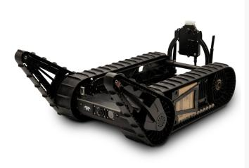
SUGV 325 represents the cutting edge in portable robotics, designed to effectively address modern challenges. With its exceptional mobility and situational awareness capabilities, this single-person-lift robot offers a versatile solution for a variety of missions. Featuring a suite of modular payloads including a highly dexterous 5-DOF manipulator, the SUGV can be tailored to meet the demands of both dismounted and mobile operations.
